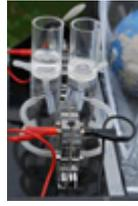
Electrolysis is a chemical reaction where water, a compound is separated into the elements Hydrogen & Oxygen by electrical means.
